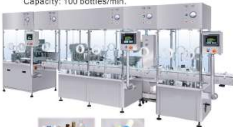
無菌充填內塞封蓋包裝線 Aseptic Filling, Stoppering & Closing Machine (Vial / Eye-Drop) Capacity: 100 bottles/min.
