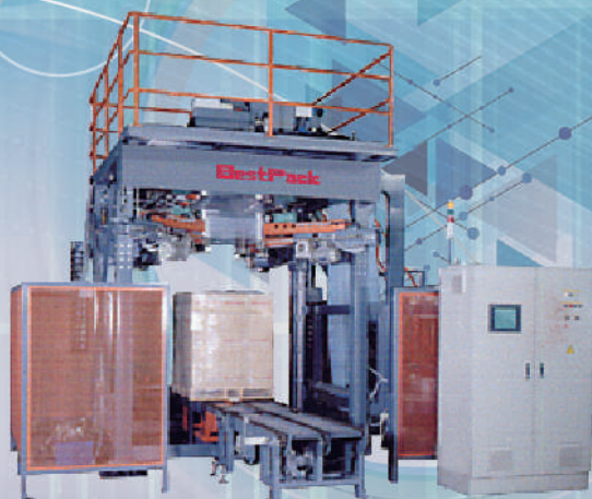
SHC2-54 冷收縮膜機 Full Protection of Pallet Loads For Transportation
