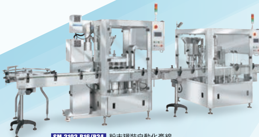
SM-2102-R16/R24 粉末罐裝自動化產線 High Speed Automatic Powder Bottle Filling Line Solution
