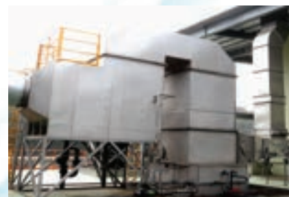
高效油霧過濾系統 High-efficiency oil mist (colloidal substance) filtration system
