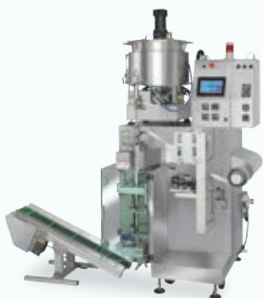
STS-01LQ-R 液體小包裝 Pump Filler with VFFS Machine - Round Corner Liquid Sachet
