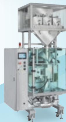
TS-2435W 顆粒大包裝 Linear Weigher with VFFS Machine - Granule Large Bag
