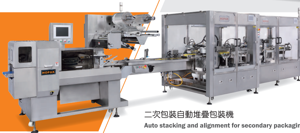
條碼檢測列印、 脫氧劑投入機整合包裝機 Bar code scanning, printing and sachet feeder packaging line (HFFS)
