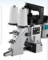
N320A 2-Thread Bag Closer for Heavy Use
