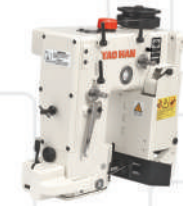
N980A (1-Needle) N980AC (For crepe or plain sew) High Speed Bag Closer
